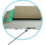
Bi-directional RS-232 interface to output the results to a printer of computer Battery compartment for the internal rechargeable battery
